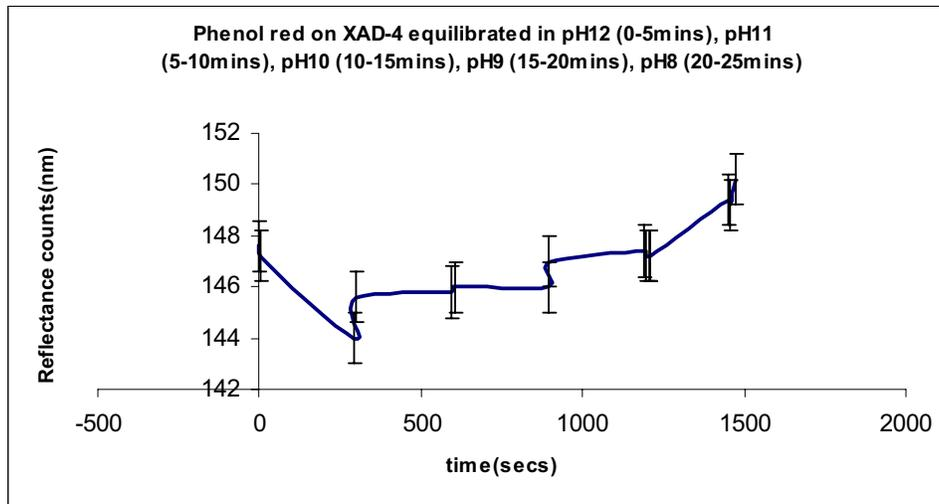
Fig 4.1.5h) XAD-4 with phenol red equilibrated in pH 12, pH 11, pH 10, pH 9 and pH 8 at 5 minutes intervals. The signal increased with decrease in buffer pH.
