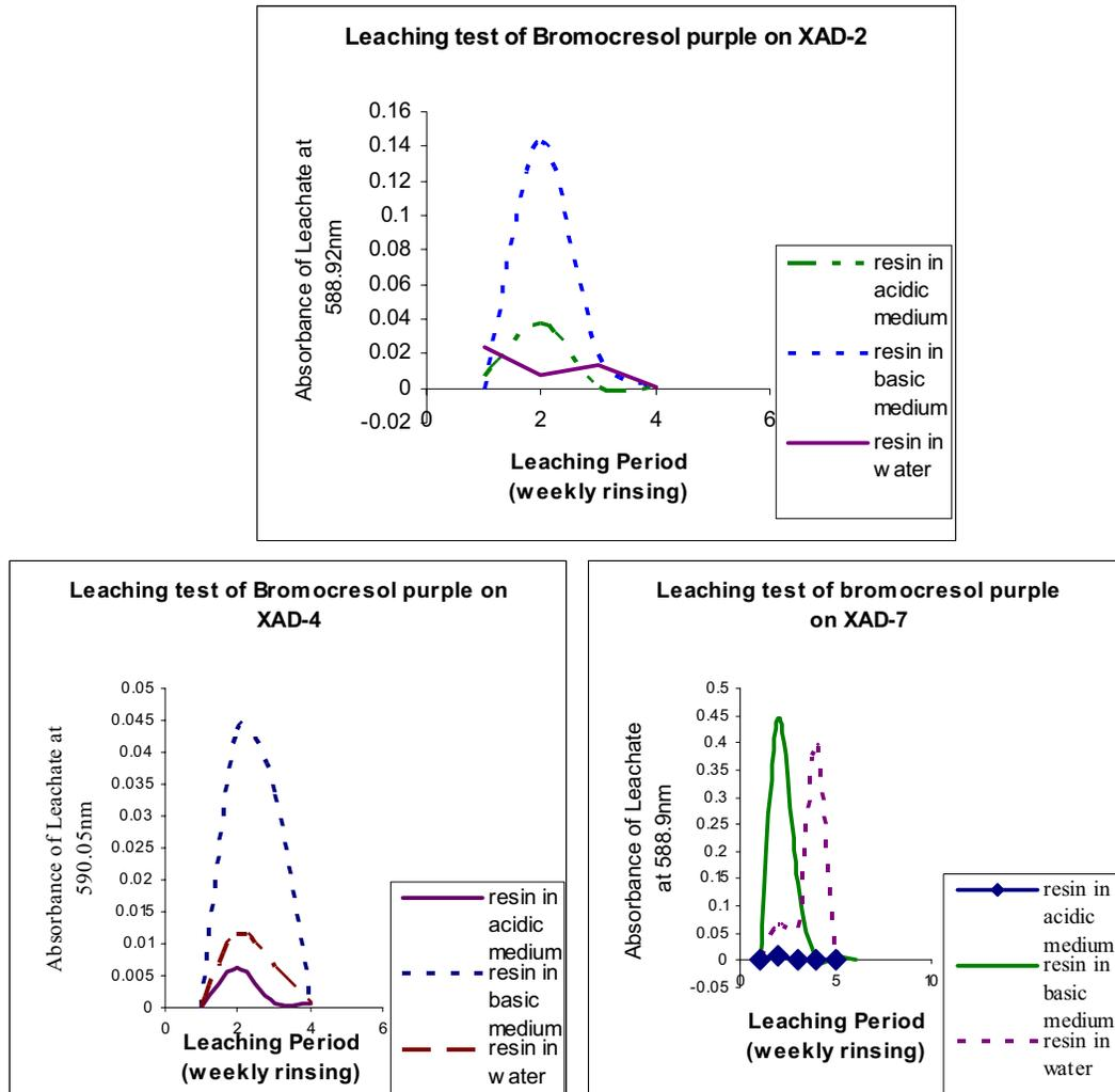
Fig 4.1.2c) Shows the absorbance of leached indicators from XAD-2, XAD-4 and XAD-7 resins placed in different pH medium. The amount of absorbance indicates the amount of the indicators leached, hence more indicators have leached in the basic medium and water.
