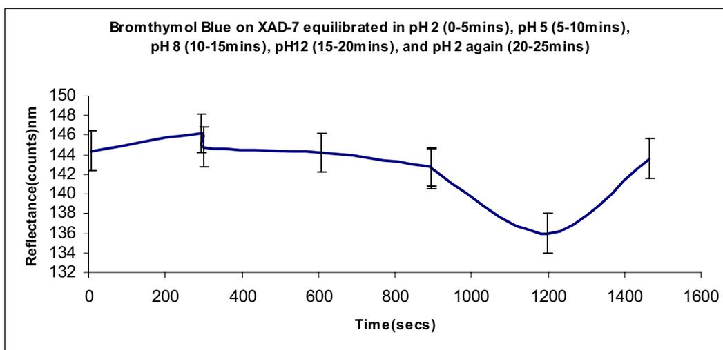
Fig 4.1.3k) XAD-7 BTB probe equilibrated in pH 2 (0-300secs), pH 5 (300-600secs), pH 8 (600-900secs), pH 12 (900-1200secs) and pH 2 (1200-1500secs). Signal increases in acidic condition and decreases in basic conditions. There was much difference in signal between pH 5-8.
