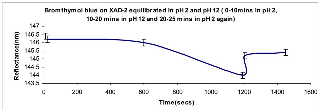
Fig 4.1.3e) shows the change in response of the XAD-2 with Bromthymol blue probe when immersed in pH 2 for first ten minutes (600secs) and in pH 12 for 10-20 minutes (600-1200secs) then again in pH 2 from 20-25 minutes (1200-1500secs).
