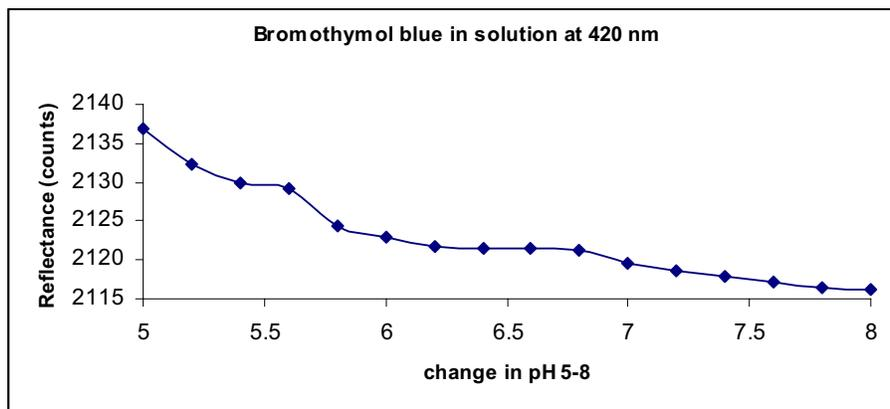
Fig 4.1.3b) shows the reflectance of indicator Bromothymol blue in buffers of pH 5.0-8.0 ( $\pm 0.2$ )
