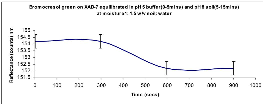
Fig 4.2.2 m) Response of bromocresol green on XAD-7 equilibrated in pH 5 buffer and pH 8 soil at moisture 1:1.5 w/v; soil : water
