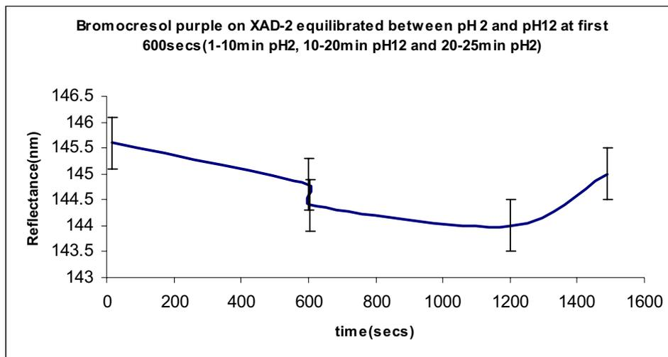
Fig 4.1.2d) shows the change in response of the XAD-2 with bromocresol purple probe when immersed in pH 2 for first ten minutes (600secs) and in pH 12 for 10-20 minutes (600-1200secs) then again in pH 2 from 20-25 (1200-1500secs).
