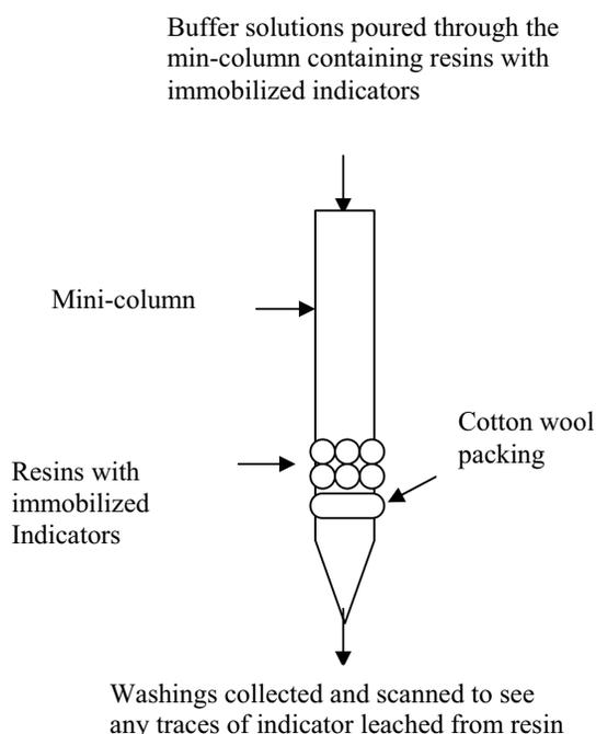
Fig 3a: Showing the set-up of the leaching test process
