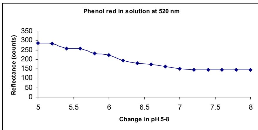
Fig 4.1.5b) shows the reflectance of indicator phenol red in buffers of pH 5.0-8.0. ( $\pm 0.2$ ).
