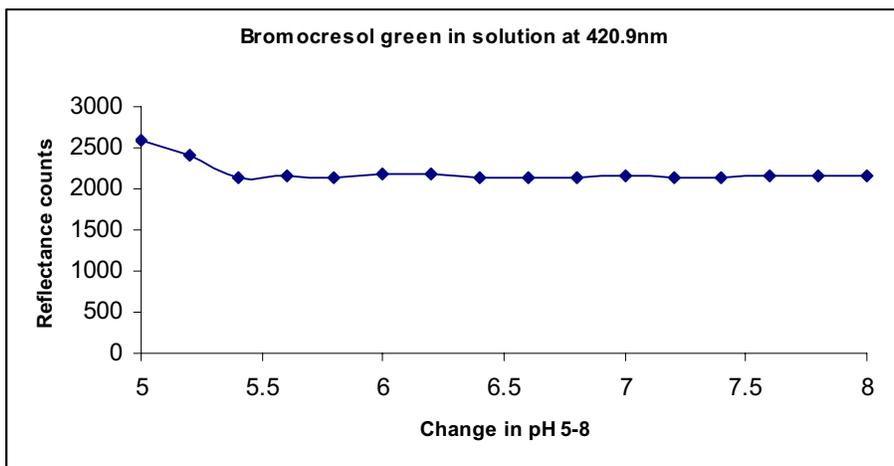
Fig 4.1.1b) Shows the reflectance of indicator bromocresol green in buffers of pH 5.0-8.0. ( $\pm 0.2$ ).
