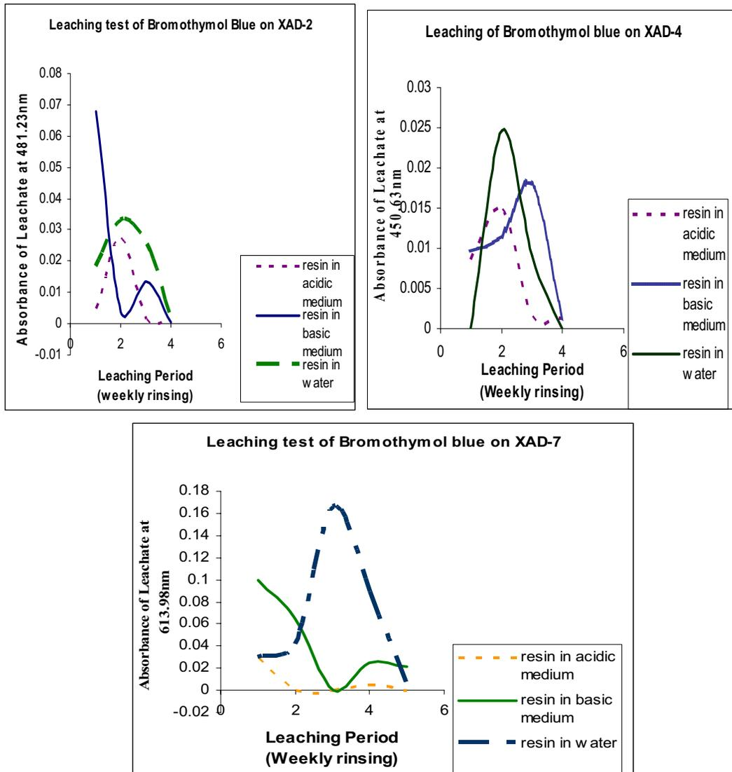
Fig 4.1.3c) shows the absorbance of leached indicators from XAD-2, XAD-4 and XAD-7 resins placed in different pH medium. The amount of absorbance indicates the amount of the indicators leached; hence more indicators have leached in the basic medium and water.
