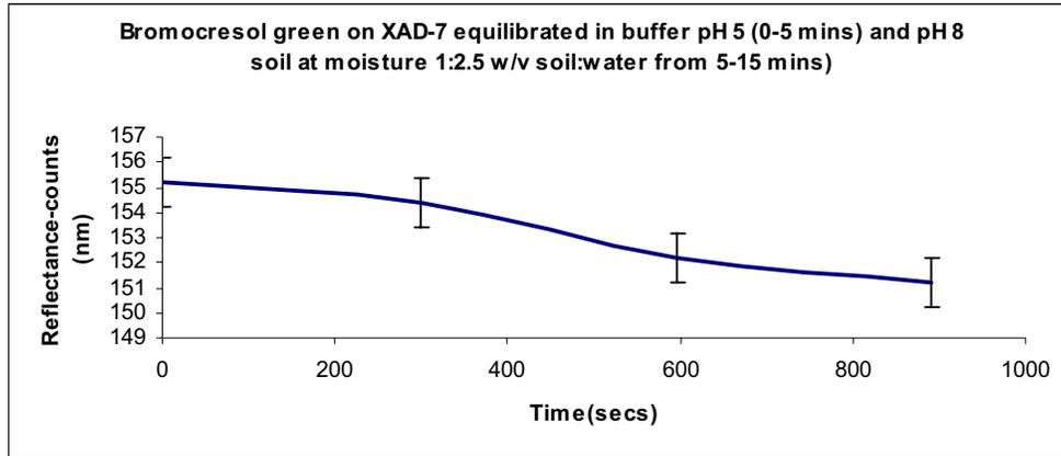
Fig 4.2.2 l) Response of bromocresol green on XAD-7 equilibrated in pH 5 buffer and pH 8 soil at moisture 1:2.5 w/v; soil : water
