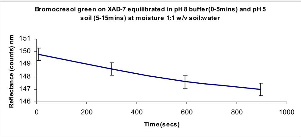
Fig 4.2.2 q) Response of bromocresol green on XAD-7 equilibrated in pH 8 buffer and pH 5 soil at moisture 1:1 w/v; soil : water
