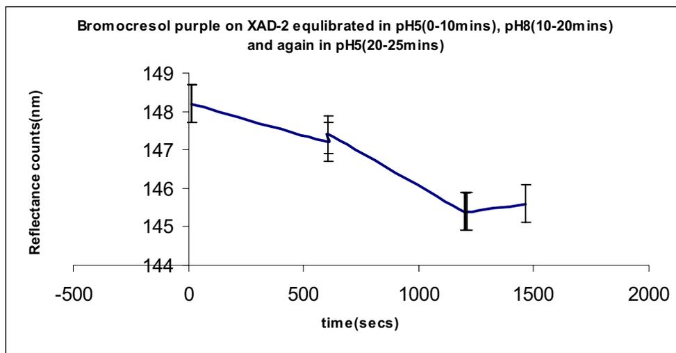
Fig 4.1.2e) the equilibration of XAD-2 bromocresol purple probe in pH 5 and pH 8 showed gradual decrease in signal with no good response with change in buffer pH.
