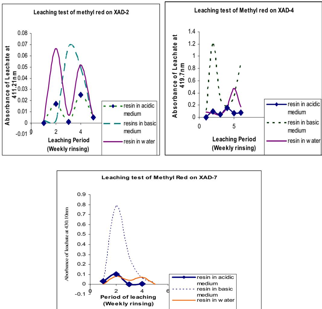
Fig 4.1.4c) shows the absorbance of leached indicators from XAD-2, XAD-4 and XAD-7 resins placed in different pH medium. The amount of absorbance indicates the amount of the indicators leached; hence more indicators have leached in the basic medium and water.
