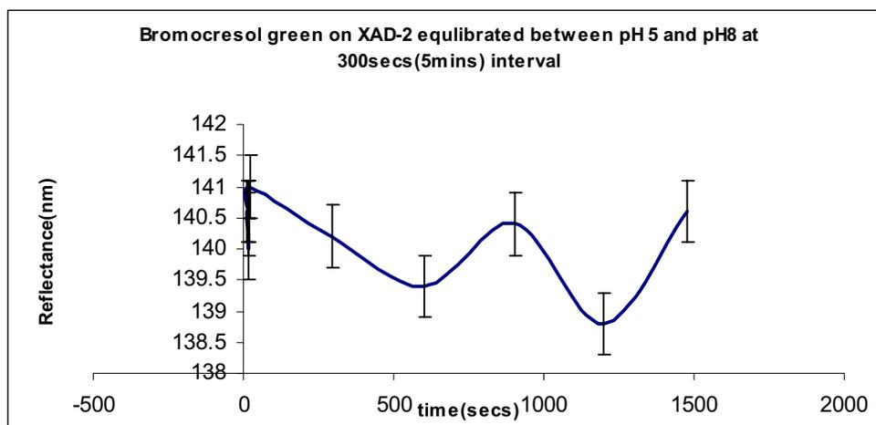
Fig: 4.1.1.d) Shows the change in response of the XAD-2 with bromocresol green probe when immersed in pH 5 and pH 8 respectively at every 5 minutes intervals.
