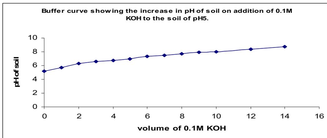
Fig 4.2.1a) shows the amount of 0.1 M KOH was added to increase the pH of soil solution (4 g in 10 ml water) from pH 5 to pH close to 8.
