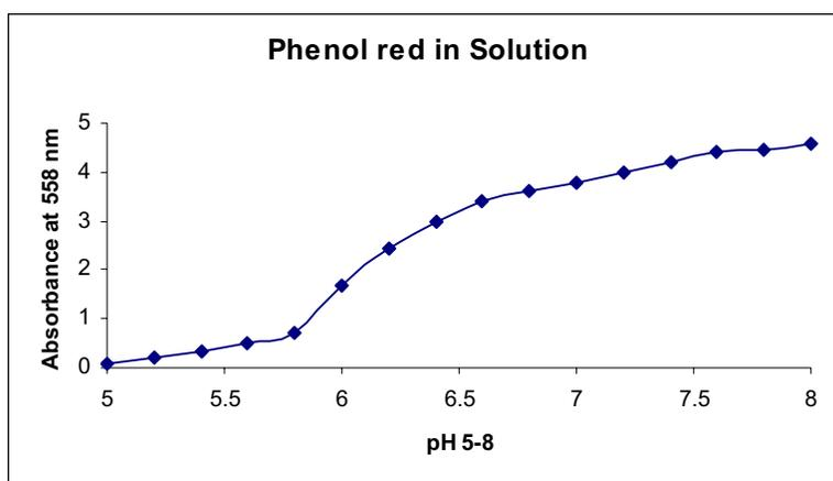
Fig 4.1.5a) shows the absorbance of indicator phenol red in buffers of pH 5.0-8.0. ( $\pm 0.2$ ) at 558nm
