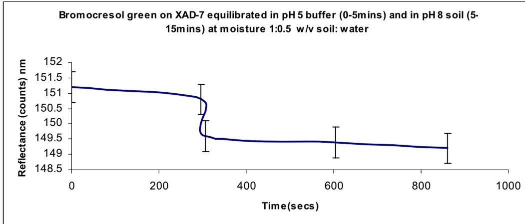
Fig 4.2.2 o) Response of bromocresol green on XAD-7 equilibrated in pH 5 buffer and pH 8 soil at moisture 1:0.5 w/v; soil : water
