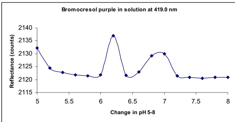
Fig 4.1.2b) Shows the reflectance of indicator bromocresol purple in buffers of pH 5.0-8.0.(±0.2)
