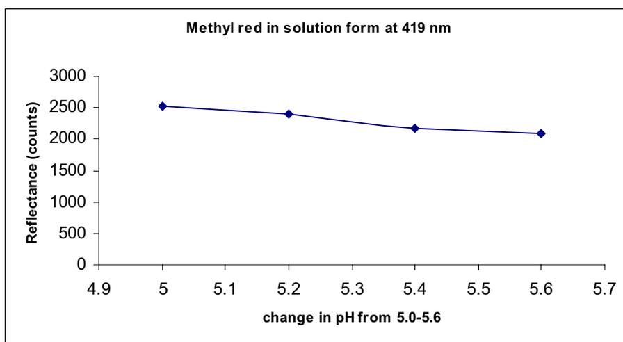
Fig 4.1.4b) shows the reflectance of indicator methyl red in buffers of pH 5.0-5.6 ( $\pm 0.2$ ).
