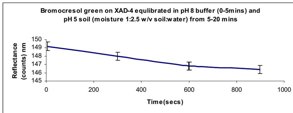
Fig 4.2.2 k) Response of bromocresol green on XAD-4 equilibrated in pH 8 buffer and pH 5 soil at moisture 1:2.5 w/v; soil : water.
