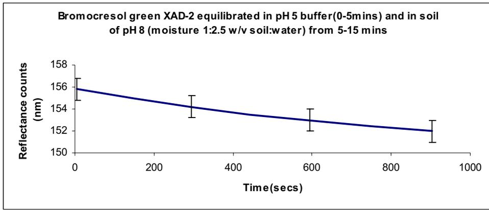
Fig 4.2.2 a) Response of bromocresol green on XAD-2 equilibrated in pH 5 buffer and pH 8 soil at moisture 1:2.5 w/v; soil : water
