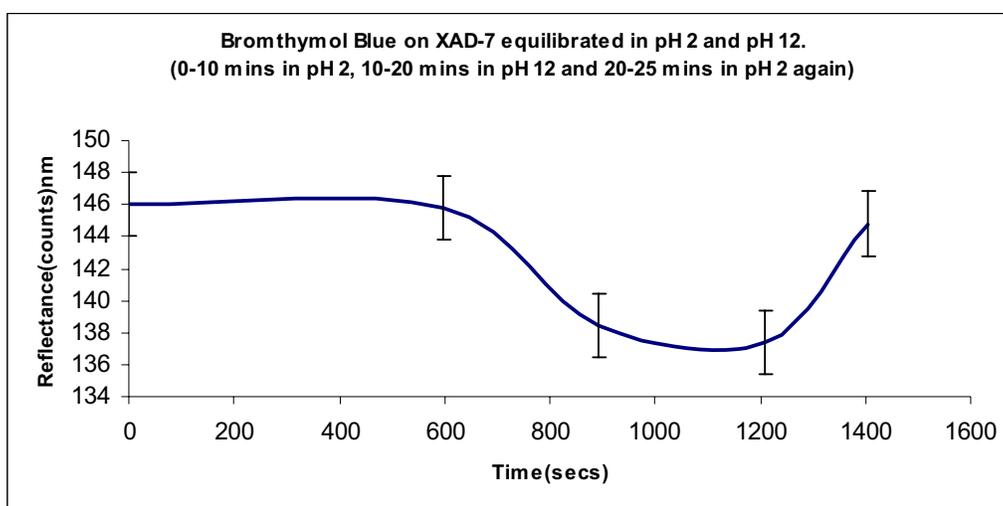
Fig 4.1.3i) XAD-7 BTB probe equilibrated in pH 2 and pH 12. Signal increases in acidic condition and decreases in basic conditions
