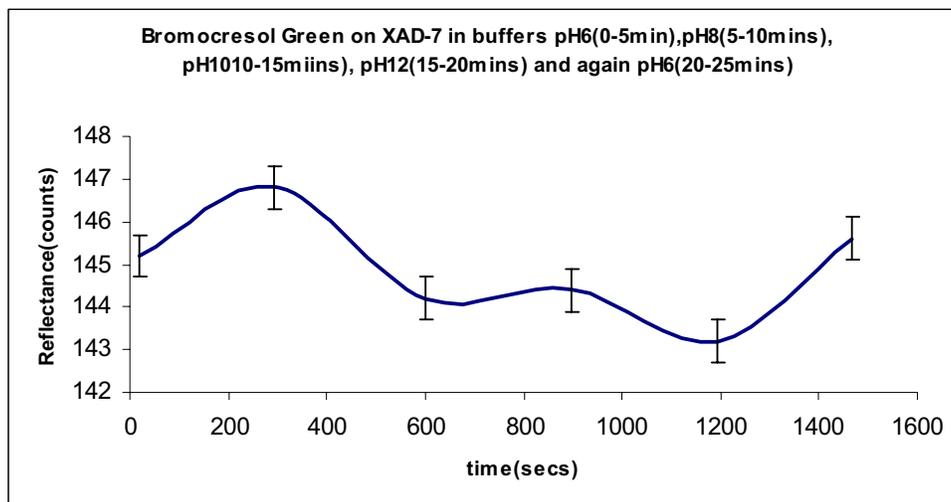
Fig: 4.1.1.h) Shows the change in response of the XAD-7 with bromocresol green probe when immersed in pH 6, pH 8, pH 10, pH 12 and again in pH 6 at 5 minutes intervals.
