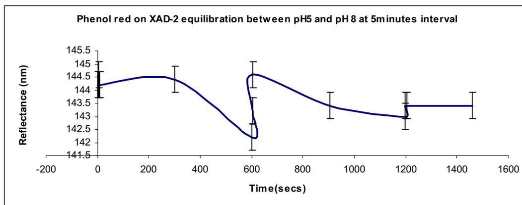
Fig 4.1.5d) shows XAD-2-phenol red probe equilibrated in pH 5 buffer (0-300secs, 600-900secs, 1200-1500secs) and pH 8 buffer (300-600secs, 900-1200secs).
