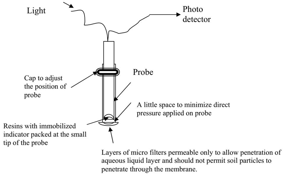
Fig 4.4.3 a) Design of probe for limiting soil particle interference.
