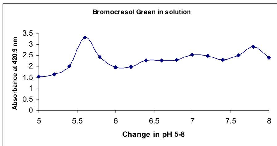
Fig 4.1.1a) Shows the absorbance of indicator bromocresol green in buffers of pH 5.0-8.0. ( $\pm 0.2$ ).
