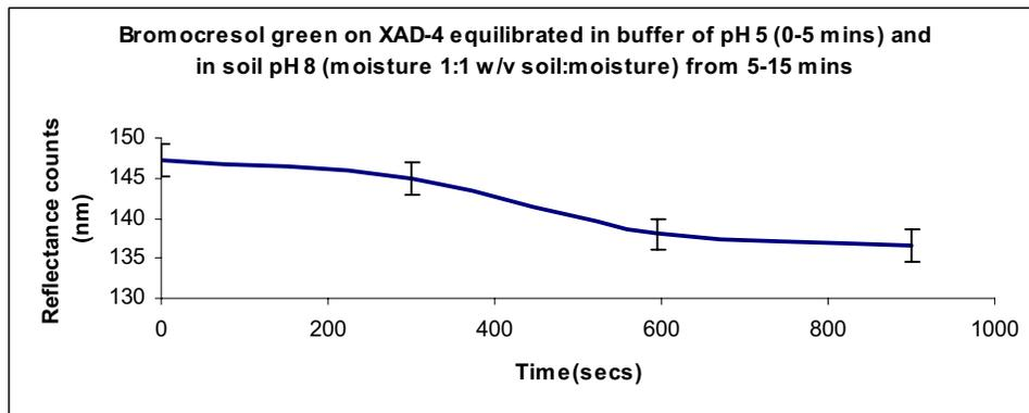
Fig 4.2.2 h) Response of bromocresol green on XAD-4 equilibrated in pH 5 buffer and pH 8 soil at moisture 1:1 w/v; soil : water
