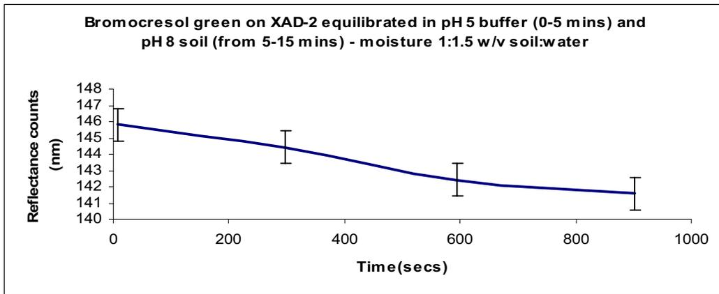
Fig 4.2.2 b) Response of bromocresol green on XAD-2 equilibrated in pH 5 buffer and pH 8 soil at moisture 1:1.5 w/v; soil : water
