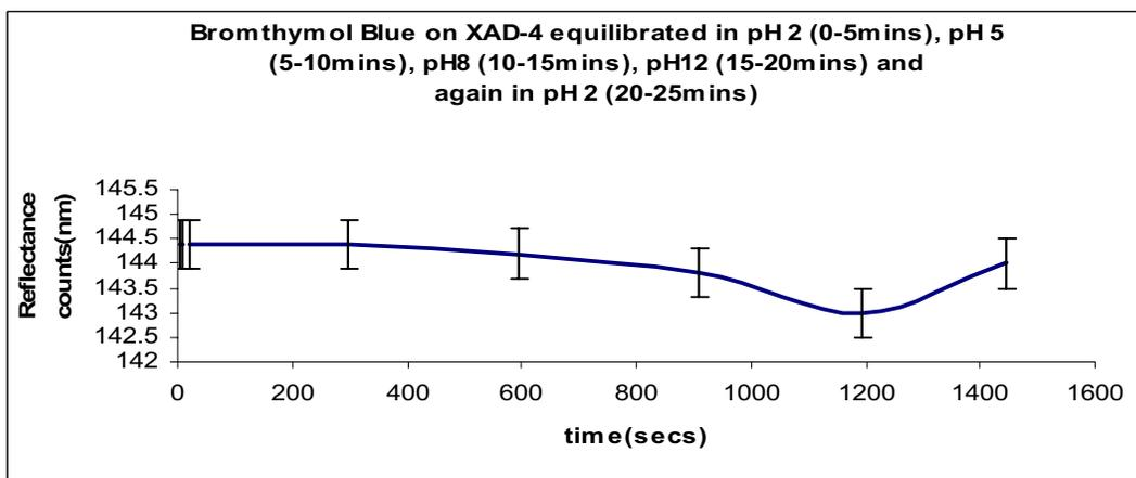
Fig 4.1.3h) shows the change in response of the XAD-4 with Bromothymol blue probe when immersed in pH 2 (0-300secs), pH 5 (300-600secs), pH 8 (600-900secs), pH 12 (900-1200secs) and again in pH 2 (1200-1500secs).
