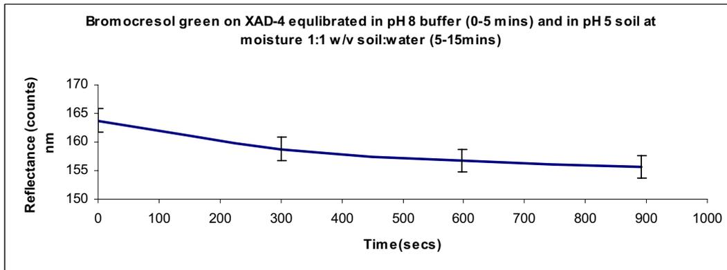
Fig 4.2.2 j) Response of bromocresol green on XAD-4 equilibrated in pH 8 buffer and pH 5 soil at moisture 1:1 w/v; soil : water
