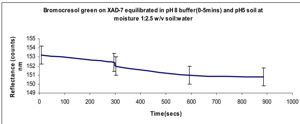
Fig 4.2.2 p) Response of bromocresol green on XAD-7 equilibrated in pH 8 buffer and pH 5 soil at moisture 1:2.5 w/v; soil : water
