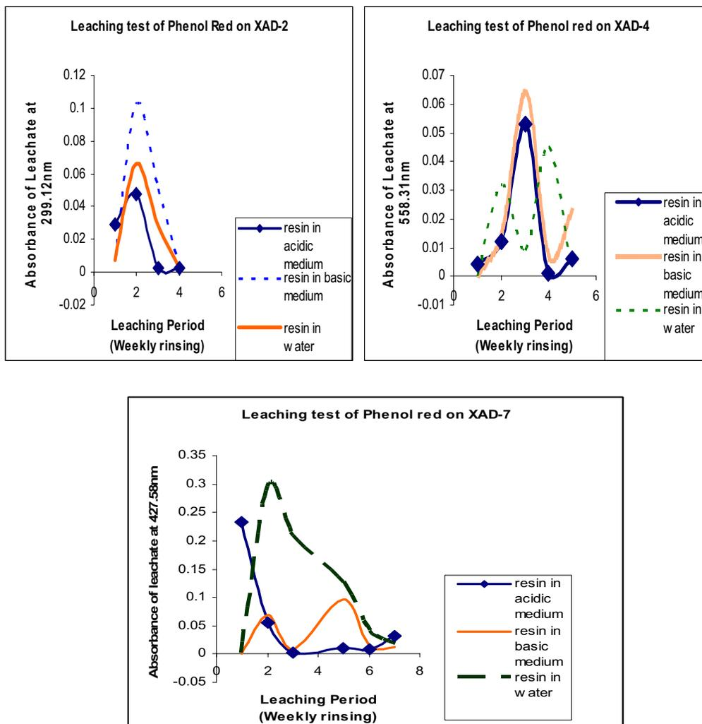
Fig 4.1.5c) Shows the absorbance of leached indicators from XAD-2, XAD-4 and XAD-7 resins placed in different pH medium. The amount of absorbance indicates the amount of the indicators leached; hence more indicators have leached in the basic medium and water.
