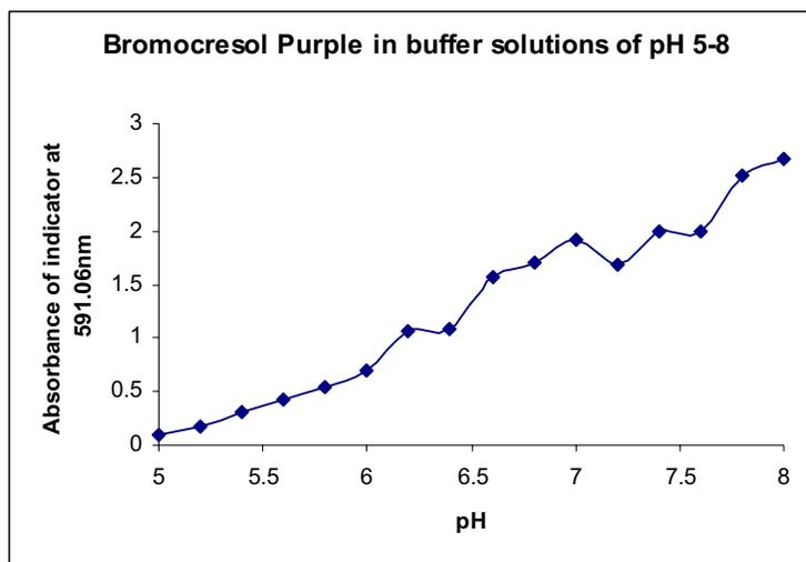
Fig 4.1.2a) Shows the absorbance of indicator bromocresol purple in buffers of pH 5.0-8.0.(±0.2)
