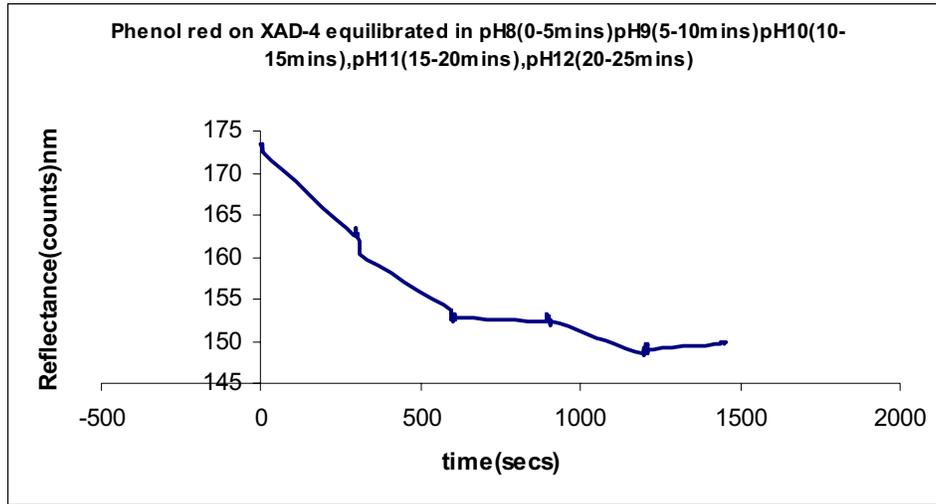
Fig 4.1.5g) XAD-4 with phenol red equilibrated in pH 8, pH 9, pH 10, pH 11 and pH 12 at 5 minutes intervals. The signal decreased with increase in buffer pH
