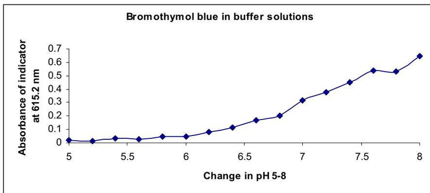
Fig 4.1.3a) shows the absorbance of indicator Bromothymol blue in buffers of pH 5.0-8.0 ( $\pm 0.2$ ).
