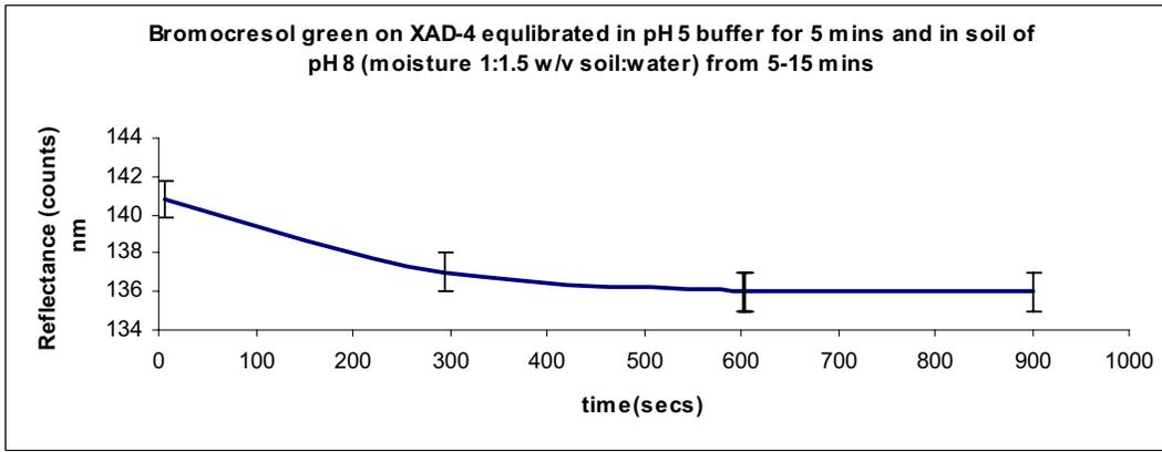
Fig 4.2.2 g) Response of bromocresol green on XAD-4 equilibrated in pH 5 buffer and pH 8 soil at moisture 1:1.5 w/v; soil : water
