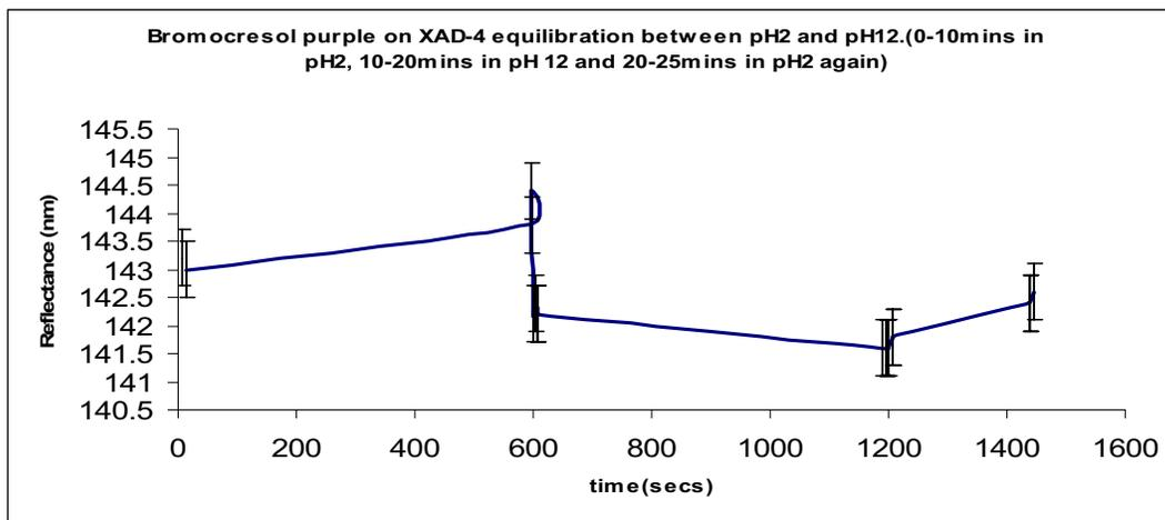
Fig 4.1.2g) shows the change in response of the XAD-4 with bromocresol purple probe when immersed in pH 2 for first ten minutes (600secs) and in pH 12 for 10-20 minutes (600-1200secs) then again in pH 2 from 20-25 (1200-1500secs)
