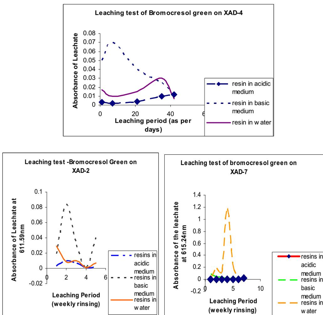
Fig: 4.1.1c) Shows the absorbance of leached indicators from XAD-2, XAD-4 and XAD-7 resins placed in different pH medium. The amount of absorbance indicates the amount of the indicators leached; hence more indicators have leached in the basic medium and water.
