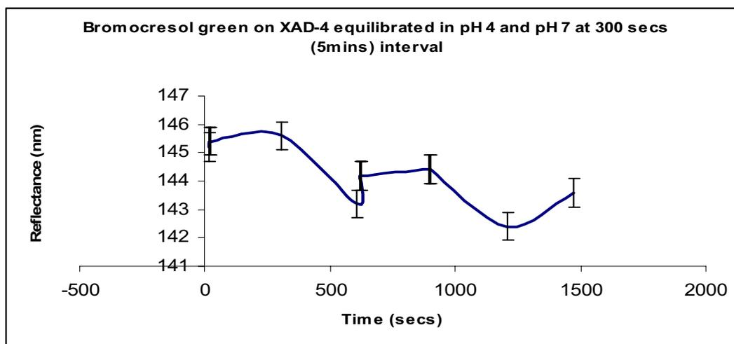
Fig: 4.1.1.e) Shows the change in response of the XAD-4 with bromocresol green probe when immersed in pH 4 and pH 7 respectively at every 5 minutes intervals.
