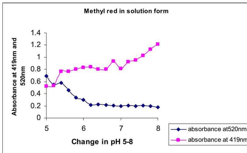
Fig 4.1.4a) shows the absorbance of indicator methyl red in buffers of pH 5.0-8.0. ( $\pm 0.2$ )
