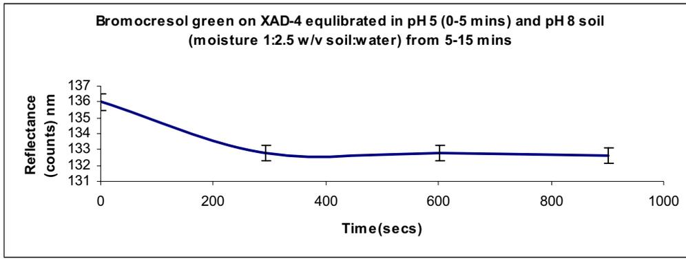
Fig 4.2.2 f) Response of bromocresol green on XAD-4 equilibrated in pH 5 buffer and pH 8 soil at moisture 1:2.5 w/v; soil : water
