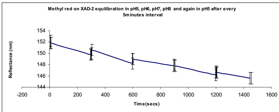
Fig 4.1.4d) The XAD-2 with methyl red equilibrated between pH 5-8. There is continuous decrease in signal both in acidic and basic conditions.
