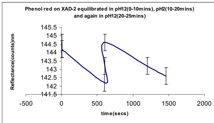
Fig 4.1.5e) shows XAD-2-phenol red probe equilibrated in pH 2 buffer (600-1200secs) and pH 12 buffer (0-10 mins, 1200-1500secs).
