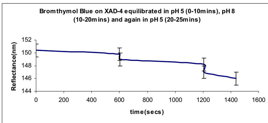
Fig 4.1.3f) shows the change in response of the XAD-4 with bromthymol blue probe when immersed in pH 8 (0-600secs), pH 5 (600-1200secs), pH 8 (1200-1500secs). It shows inverse response in acidic and basic condition.
