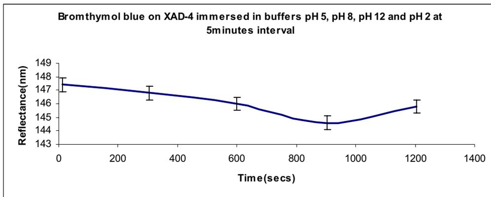
Fig 4.1.3g) shows the change in response of the XAD-4 with Bromothymol blue probe when immersed in pH 5 (0-300secs), pH 8 (300-600secs), pH 12 (600-900secs) and in pH 2 (900-1200secs).
