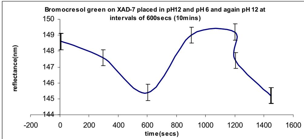
Fig: 4.1.1.f) Shows the change in response of the XAD-7 with the bromocresol green probe when immersed in pH12 and pH 6 respectively at every ten minutes (600secs) intervals.
