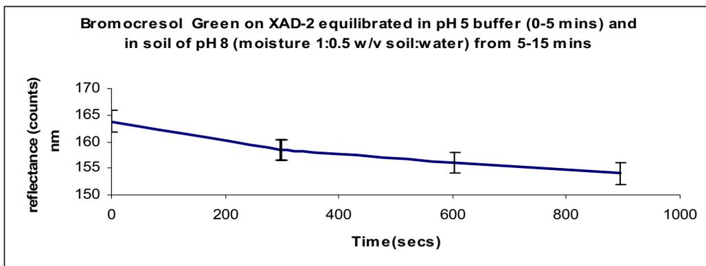
Fig 4.2.2 d) Response of bromocresol green on XAD-2 equilibrated in pH 5 buffer and pH 8 soil at moisture 1:0.5 w/v; soil : water
