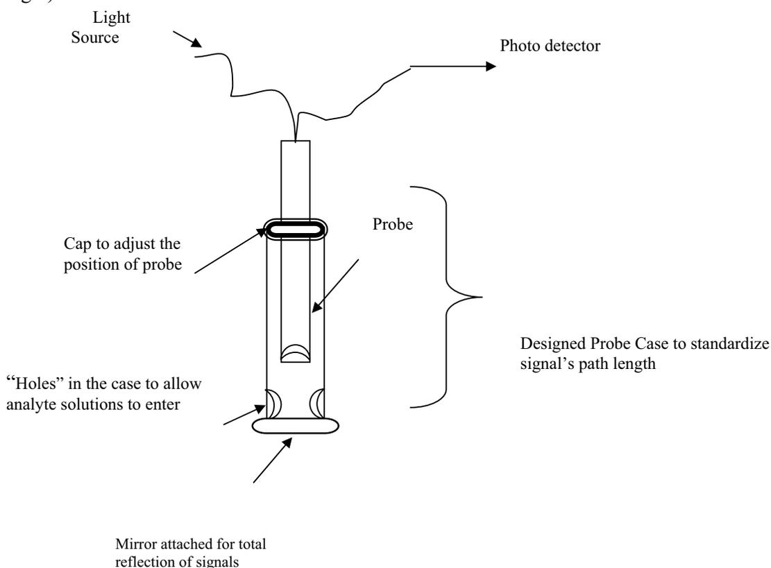
Fig 4.4.1 a) Design of probe set-up for standardization of signal at equal path length.
