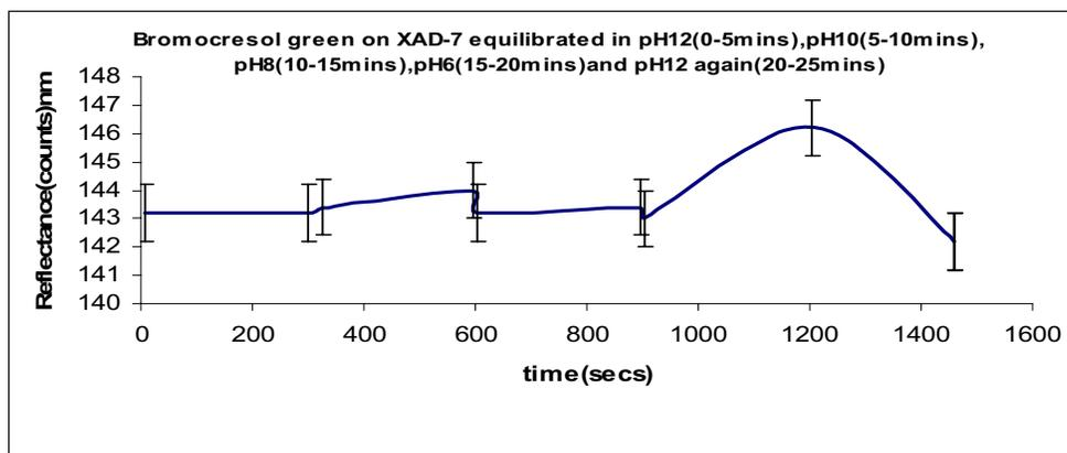
Fig:4.1.1.g) Shows the change in response of the XAD-7 with bromocresol green probe when immersed in pH 12, pH 10, pH 8, pH 6 and again in pH 12 at 5 minutes intervals.
