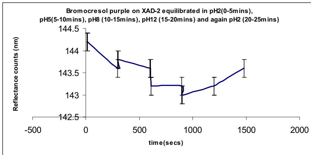
Fig 4.1.2f) shows response of XAD-2 bromocresol purple probe immersed in pH 2, pH 5, pH 8 and pH 12. There wasn't much difference in signal from pH 5-8.
