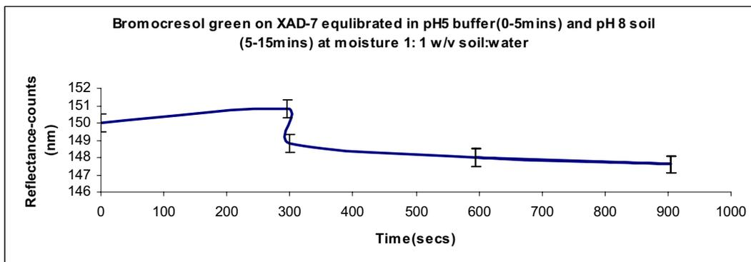
Fig 4.2.2 n) Response of bromocresol green on XAD-7 equilibrated in pH 5 buffer and pH 8 soil at moisture 1:1 w/v; soil : water
