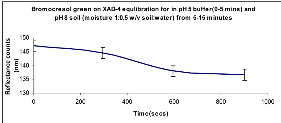
Fig 4.2.2 i) Response of bromocresol green on XAD-4 equilibrated in pH 5 buffer and pH 8 soil at moisture 1:0.5 w/v; soil : water
