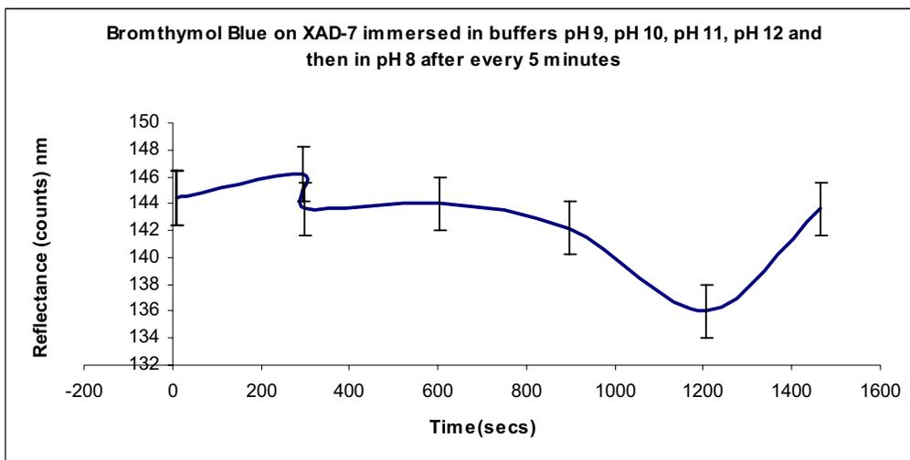
Fig 4.1.3j) XAD-7 BTB probe equilibrated in pH 9 (0-300secs), pH 10 (300-600secs), pH 11 (600-900secs), pH 12 (900-1200secs) and pH 8 (1200-1500secs). Signal increases in acidic condition and decreases in basic conditions
