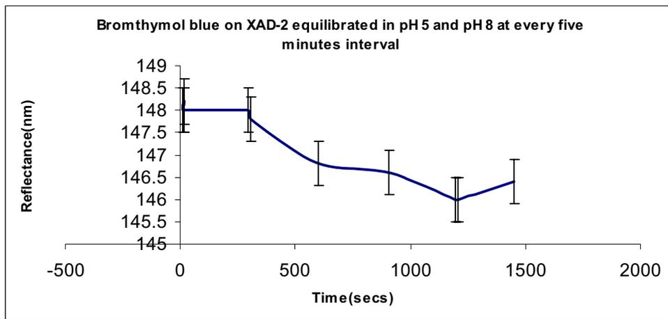
Fig 4.1.3d) shows the response of BTB-XAD-2 probe equilibrated in pH 8(0-300secs, 600-900secs, 1200-1500secs) and pH 5(300-600secs, 900-1200secs). There wasn't much difference in signal with change in pH of buffers.
