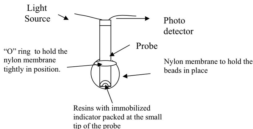
Fig 3b: Showing the design of the fiber optic pH probe.
